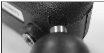
Figure 6: Using the test light magnet to reset the R7 Receiver
