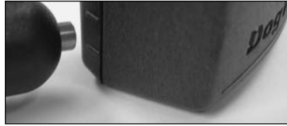
Using the test light magnet to reset the R1200 Receiver
