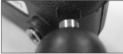
Using the test light magnet to reset the R1200m Receiver
