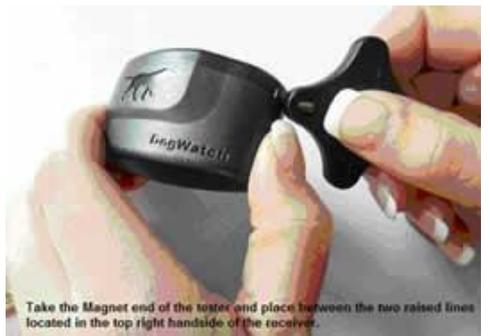
**If the collar is not beeping through the levels** this means there is a battery issue. Ensure the battery is put in the correct way: 3.0v battery for the mini collars needs to be **+ end up** & 3.6v battery for the standard collars need to be **+ end down**. Make sure the battery cap is on securely and re-test the collar with the tester. If it still doesn't work put a new battery in the collar, which can be ordered from our [shop](#).
